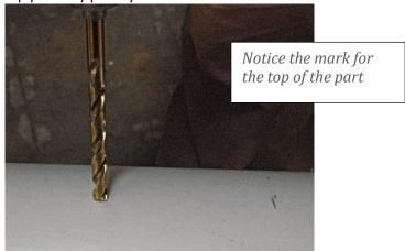
Figure 3 -- Drilling Pilot Hole
